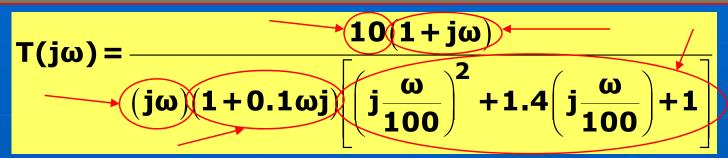
Identify the basic factors and corner frequencies : -Constant gain K : K=10, 20log10=20 [dB] -First order factor (simple lead - real zero) : T=1 ( $\omega_{c1}=1/T=1$ ) - for magnitude plot -Integral factor :  $1/j\omega$ -First order factor (simple lag – real pole) :  $T=0.1 (\omega_{c1}=1/T=10) - for magnitude plot$ -Quadratic factor (complex conjugate poles) :  $\omega_n = \omega_{c1} = 100, \xi = 0.7 - for magnitude plot$
