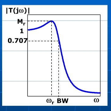
BW is directly proportional to on and gives an indication of the transient response characteristics of a control system. The larger the bandwidth is, the faster the system responds.
