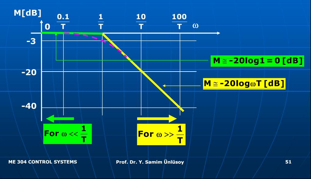
**ω<sub>c</sub>=1/T** is called the corner (break) frequency. Maximum error between the linear approximation and the exact value will be at the corner frequency.
