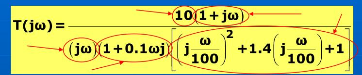
Identify the basic factors and corner frequencies : -Constant gain K : K=10, 20log10=20 [dB] -First order factor (simple lead – real zero) : T=1 (ω<sub>c2</sub>=0.1/T=0.1, ω<sub>c3</sub>=10/T=10) – for phase plot -Integral factor : 1/jω -First order factor (simple lag – real pole) : T=0.1  $(\omega_{c2}=0.1/T=1, \omega_{c3}=10/T=100) - for phase plot$ -Quadratic factor (complex conjugate poles) :  $\omega_n = 100$  $(\omega_{c2}=\omega_{n}/10=10, \omega_{c3}=10\omega_{n}=1000) - for phase plot$
