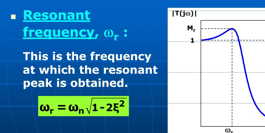
Note that resonant frequency is different than both the undamped and damped natural frequencies!
