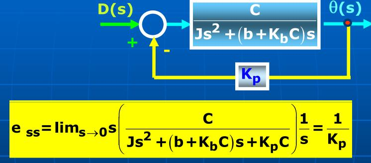
It is observed that for minimum steady state error due to a step disturbance, and a ramp input, K<sub>p</sub> must be as large as stability requirements allow.
