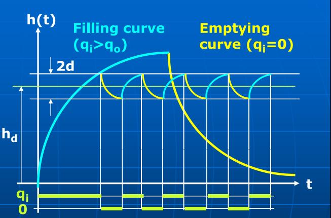
Then the solenoid valve will be shut off until the water level drops below the desired level by half the differential gap. The water level will continuously oscillate about the desired level.
