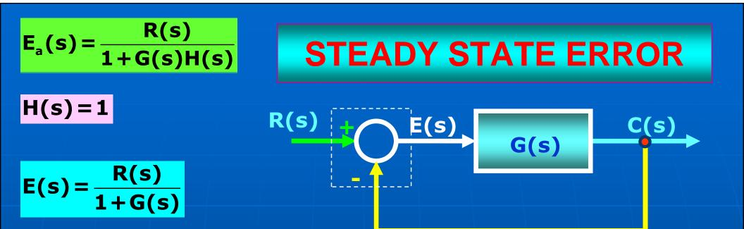
Note that the actuating and actual errors will be identical only for a unity feedback system, i.e. with an ideal sensor.
