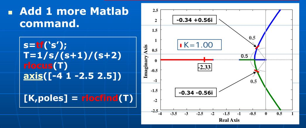
Click on the crosshair cursor in the graphics window put by rlocfind to select a pole location on an existing root locus. The root locus gain associated with this point is returned in K and all the system poles for this gain are returned in poles.
