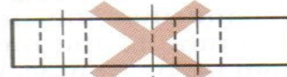
POOR Holes not symmetrical
