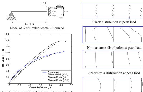
Analytical results without shear with and without tensile strength, with shear and tensile strengths vs. experiment
